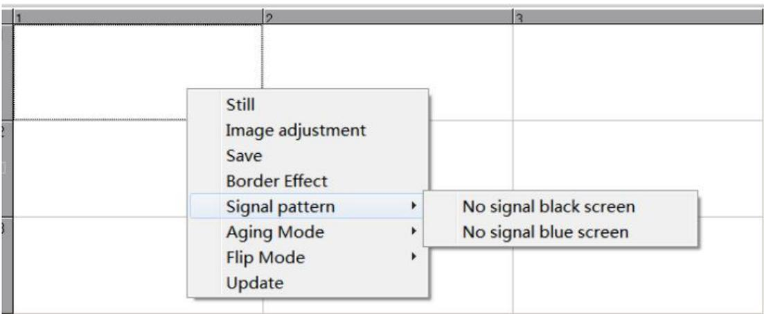
"Signal pattern" is to deal with the state of the screen with no-signal;
