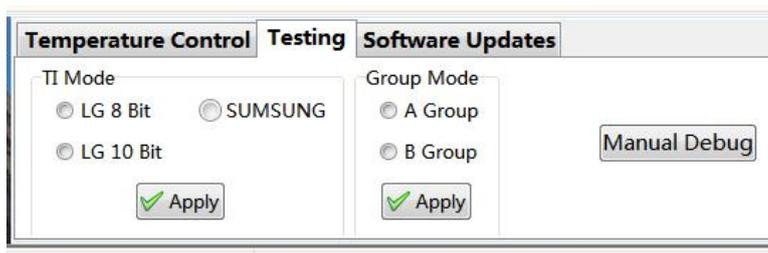
“Testing” is mainly for panel parameter adjustment. “Ti Mode” is the output signal format of image processor,
