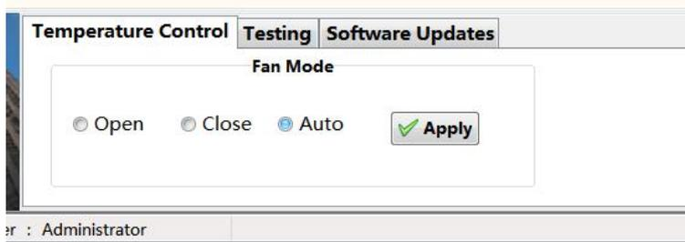
When use Temp. Control, you can choose “Auto” to recognize temperature automatically or “Manualsetting” to set the RunValue & StopValue, or choose “Open” / “Close” to keep on /off status, multiple combination provide much convenience for users.
