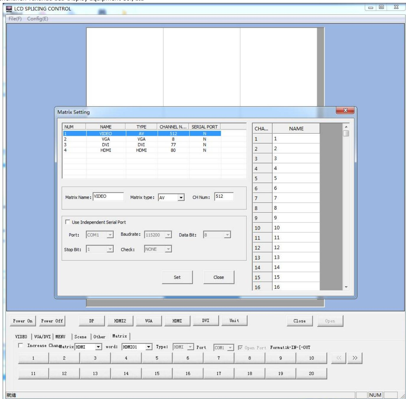
On the right side of the options menu, you can edit the matrix button input channel name, set the number of matrix input channels and select to open the corresponding type of matrix serial port.
