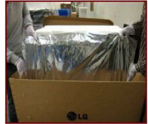
One hand holds AI bag open area, the other hand guides LCM.
