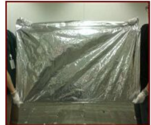
Shift LCM to target place in vertical status by two operators.
