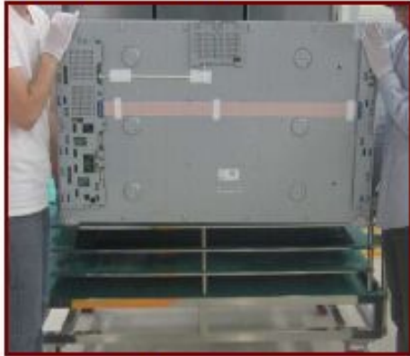
Move LCM in vertical status to prevent LCM bent.
